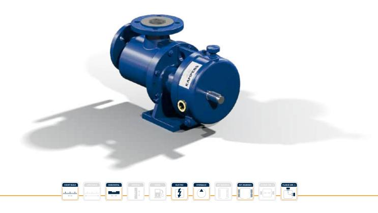
KAMPERS 1M-series LHE is constructed with one pair of screws which makes it suitable for smaller capacities. Gears and bearings are placed on one side making the pump casing easy to remove for cleaning. The screw entrance is inline with the suction flange, resulting in a compact design and low NPSHr values. The pump is self-priming and can handle limited dry-running. In LHE.S execution it can handle corrosive fluids as well.
